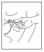
Reinstall the wheel nuts with the cone-shaped end of the nuts toward the wheel. Tighten each nut by hand until the wheel is held against the hub.
